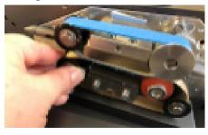
Push the lower of the two guiding rollers to the right against the spring to release the tension for the lower Teflon belt.
