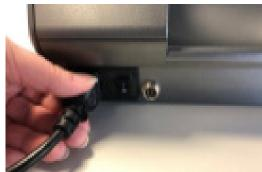
Disconnect power to the machine by removing the power cord completely from the machine.
