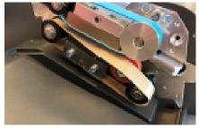
Remove the slackened Teflon belt from the rollers.
