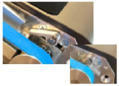
Turn the tension lever to move the transport rolls apart.
