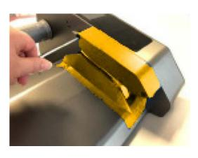
Undo both screws of upper cover with appropriate hex key and remove cover.
