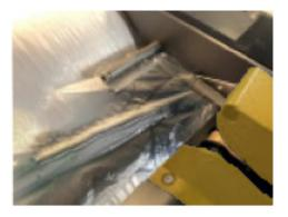
Thread the film through the pins and over the airpipe. Start production.
