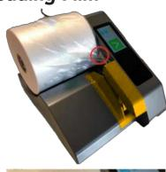
Fully seat the roll of film onto the film roll shaft. There is an air channel on one edge of the roll. The channel must be on the side closest to the machine. The correct orientation is also indicated by an arrow on the new roll of film.
