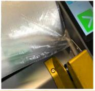
Guide the air fill channel of the film onto the blow tube. Slide the film on the blow tube.
