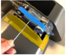
Undo the locating screw with the provided hex key.
