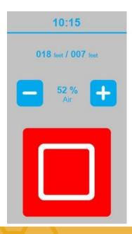
Once machine is powered on, the sealing unit will begin to heat up. When target temperature is achieved the "Start panel" will change to green and machine is ready to use.
