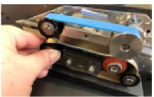
And press the roll again to the right against the spring until the Teflon belt can be placed on the right roll.
