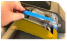
Now press the left roll to the right against the spring until it is possible to place the transport belt on the left roll.
