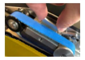
Insert the knife into the slot at the machine.
