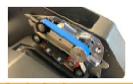
**Step 3: Loosen transport rolls**
