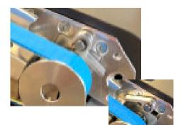
Turn the tension lever back to the left to press the transport rolls against each other.
