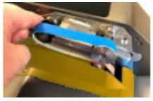
Push the upper left guiding rollers to the right against the spring to release the tension for the transport belt.
