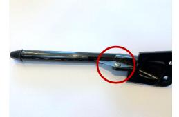
**Step 4:** Using the hex key to unscrew the screws of blade and change it.
